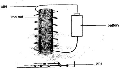
Which of the following(s) should he do to increase the number of pins that the electromagnet can attract?
